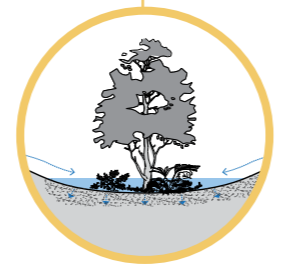
Garden beds with deep friable soils can help to slow, filter and collect water
